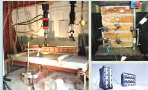
Large scale structural beam testing
